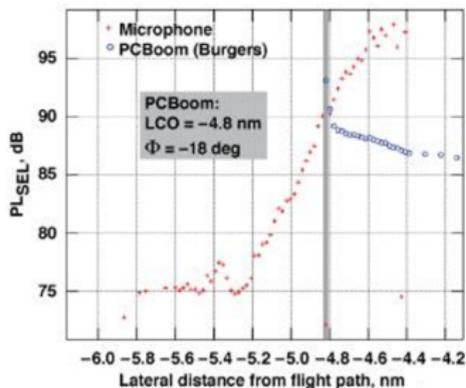
**Figure 1:** Perceived Sound Exposure level at the lateral extent of the carpet (Cliatt et al. [1]) compared with PCBoom predictions. Both figures from Cliatt et al. [1].
