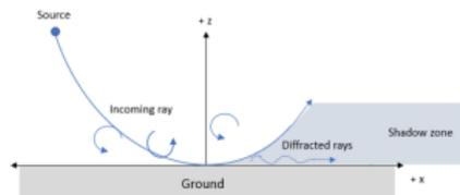
**Figure 2:** Diagram of diffraction process between incoming ray and ground
