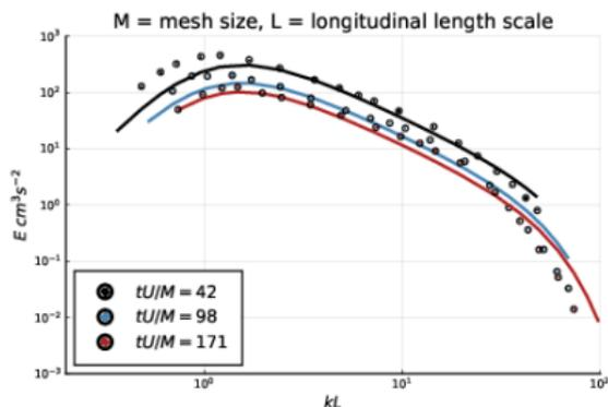
(a) Turbulent kinetic energy spectrum
