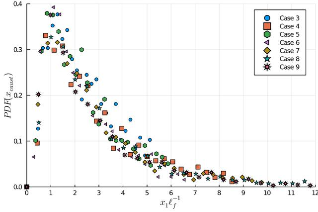
FIG. 5. Probability density functions of the first occurrence of a caustic  $P(\Delta p > 1.5\Delta p_{\text{nom}})$ , computed from simulations, along the scaled propagation distance  $x_1\ell_f^{-1}$ .
