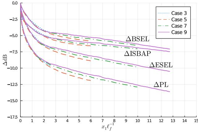
FIG. 13. Mean values of  $\Delta\text{PL}$ ,  $\Delta\text{ISBAP}$ ,  $\Delta\text{BSEL}$ , and  $\Delta\text{ESEL}$  for the N-wave.
