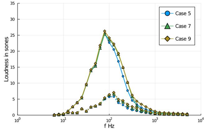
FIG. 10. Average loudness levels in sones at  $x_1\ell_f^{-1} = 5$  for the N-wave (solid lines) and low-boom waveform (dotted lines).
