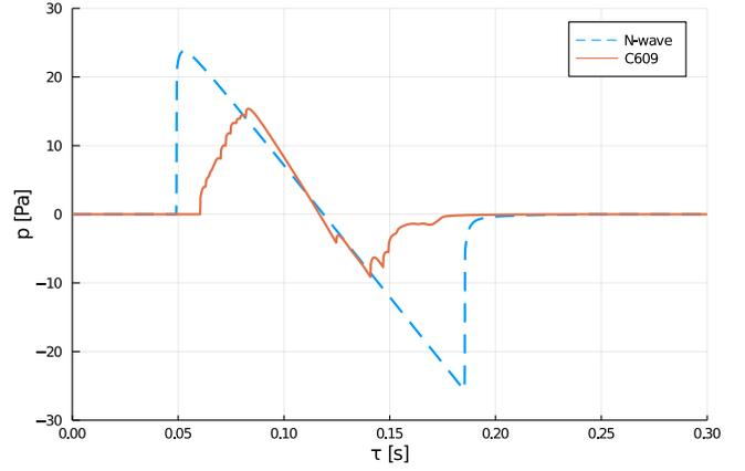
FIG. 2. The two initial waveforms considered, prescribed at the  $x_1 = 0$  plane. The N-wave (dashed line), and the simulated low-boom waveform from the NASA X-59 C609 aircraft (solid line). Both waveforms shown in the figure have been propagated by PCBoom<sup>40</sup> to just above the atmospheric boundary layer region.
