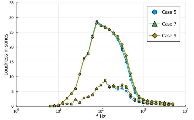
FIG. 9. Average loudness levels in sones at  $x_1\ell_f^{-1} = 1$  for the N-wave (solid lines) and low-boom waveform (dotted lines).
