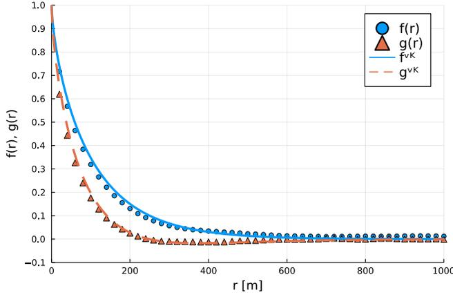
FIG. 3. Comparison of the average computed longitudinal (circles) and lateral (triangles) correlations for all 25 fields with  $u_{\text{rms}} = 1.04$  m/s and  $L_f = 106.2$  m compared to the correlation functions of the von Kármán model (solid and dashed lines).
