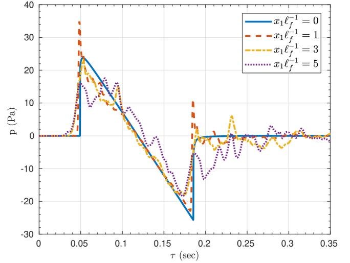
FIG. 6. Sample waveforms at different  $x_1\ell_f^{-1}$  locations for case 6 of the N-wave simulations.
