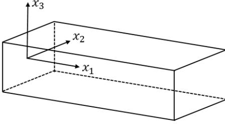
FIG. 1. Domain and coordinate system of the sonic boom simulations
