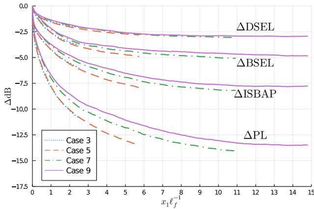
FIG. 14. Mean values of  $\Delta\text{PL}$ ,  $\Delta\text{ISBAP}$ ,  $\Delta\text{BSEL}$ , and  $\Delta\text{DSEL}$  for the low-boom waveform.
