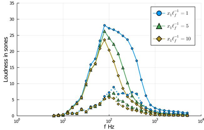
FIG. 8. Average loudness levels for the one-third octave bands in sones at case 9 for the N-wave (solid lines) and low-boom waveform (dotted lines).
