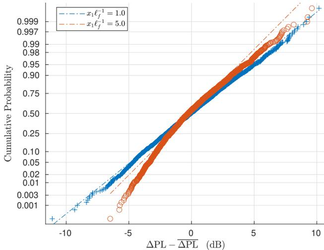
FIG. 11. Probability plots of  $\Delta\text{PL}$  with respect to the average for case 9 of the N-wave simulations.
