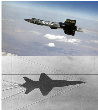
Figure 1: X-15 hypersonic aircraft (top) [1] and shadowgraph of wind tunnel model (bottom) [2].
