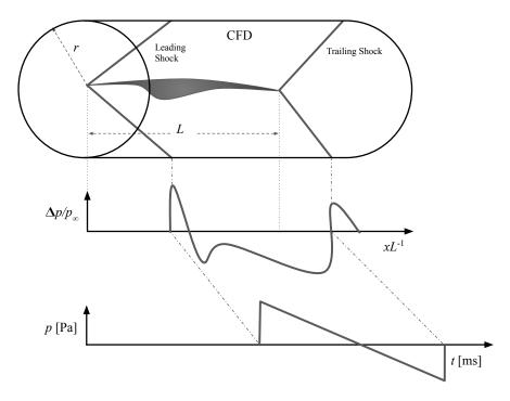
Fig. 1 Geometry, source cylinder, near-field pressure, and sonic boom signature.
