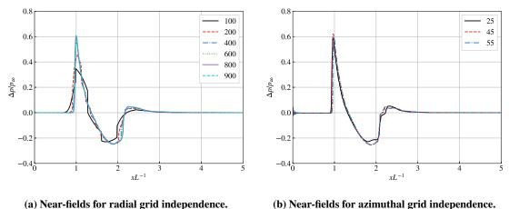
Fig. 7 Near-field extraction at  $rL^{-1} = 0.20$  for viscous reacting flow at  $M_{\infty} = 6.0$ .
