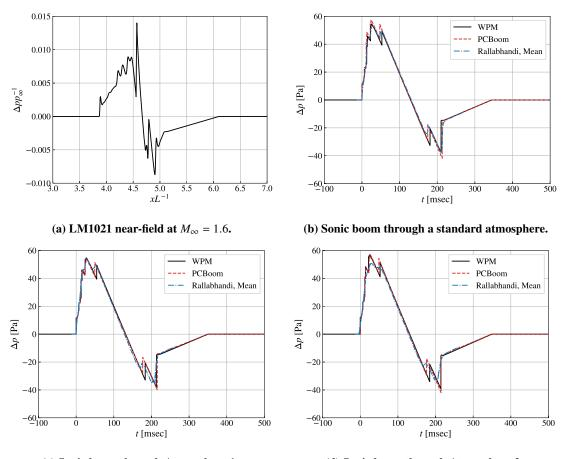
(c) Sonic boom through Atmosphere 1. (d) Sonic boom through Atmosphere 2.
