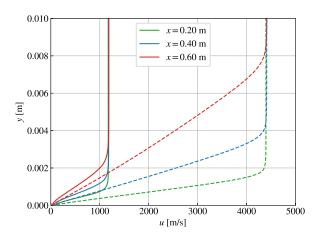
Fig. 16 Boundary layer velocity profiles of the Sears-Haack geometry at  $M_{\infty} = 4.0$  (solid lines) and  $M_{\infty} = 15.0$  (dashed lines).
