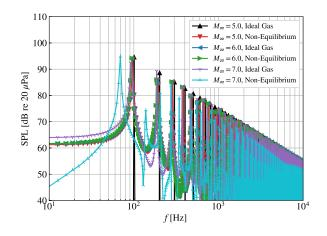
Fig. 22 SPL of the power-law waverider sonic boom signature.
