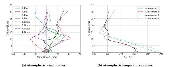
Fig. 3 Measured atmospheric profiles for sonic boom propagation validation.
