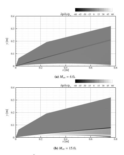
**Fig. 15** Numerical schlieren,  $\frac{1}{\rho_{\infty}} \frac{\partial \rho}{\partial y}$ , of Sears-Haack geometry at  $M_{\infty} = 4.0$  (top) and  $M_{\infty} = 15.0$  (bottom).
