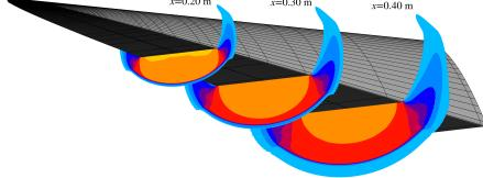
Fig. 20 Contours of  $p_{\infty}$ -normalized change in static pressure for the power-law waverider at  $M_{\infty} = 7.0$  for inviscid flow.
