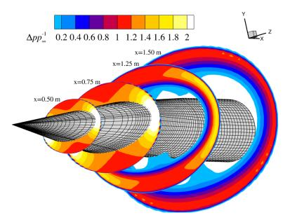
Fig. 17 Contours of  $p_{\infty}$ -normalized change in static pressure for the HIFiRE-5 geometry at  $M_{\infty} = 6.0$  for inviscid flow.
