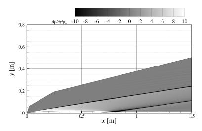
Fig. 8 Numerical schlieren,  $\frac{1}{\rho_{\infty}} \frac{\partial \rho}{\partial y}$ , of Sears-Haack geometry at  $M_{\infty} = 7.0$  for viscous flow.
