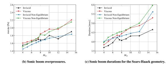
Fig. 13 Hypersonic near-field  $(rL^{-1} = 0.3937)$  and sonic boom trends for the Sears-Haack geometry.
