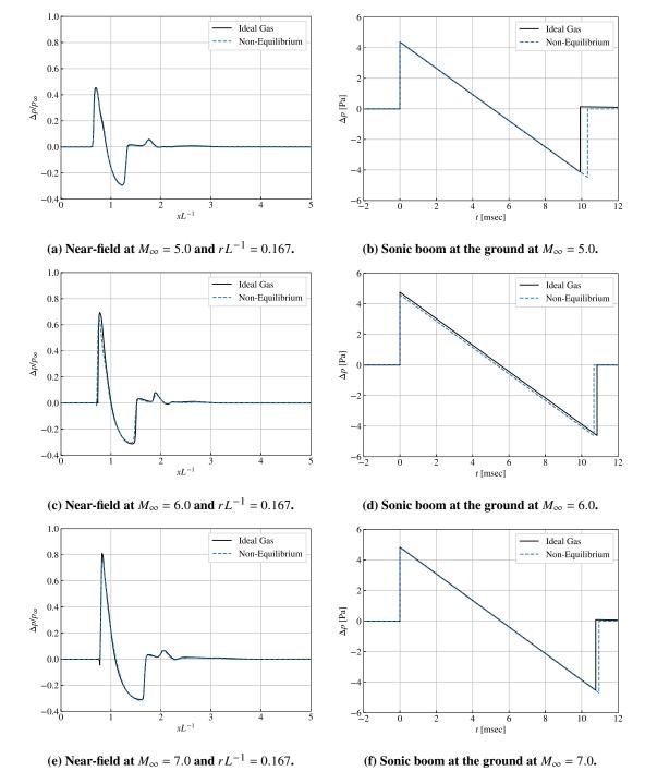
Fig. 21 Near-field predictions (left) and sonic boom predictions (right) for power-law waverider.
