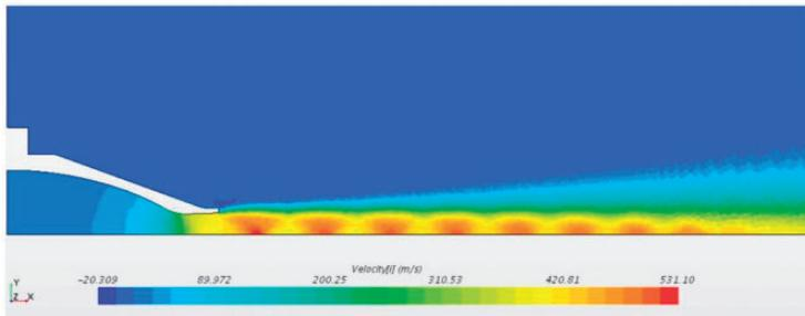
**Figure 3.** Contours of velocity component  $\bar{u}$  from an off-design supersonic jet (moving left to right).
