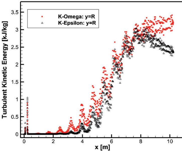
**Figure 6.** An example of the CFD portion of the homework assignments. Comparisons of two different Reynolds-averaged Navier–Stokes models.
