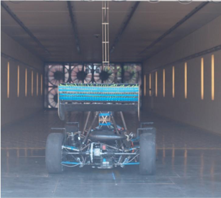
**Figure 1.** The UF formula SAE car undergoing wind-tunnel testing after its aerodynamics package is optimized with CFD.
