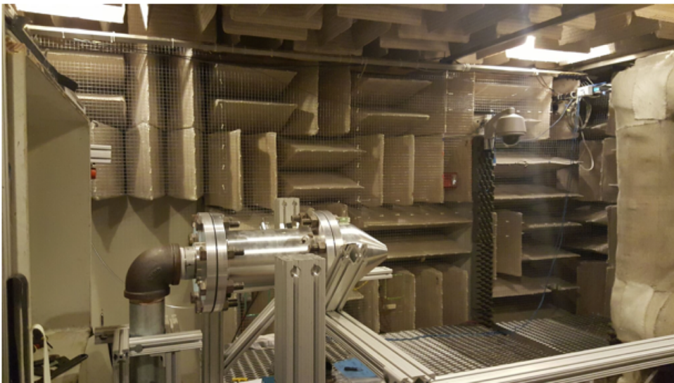
Prof. Ukeiley's - Unsteady Fluid Dynamics Group Anechoic Chamber with installed nozzle for studying jet turbulence and acoustics located in MAE-A.
