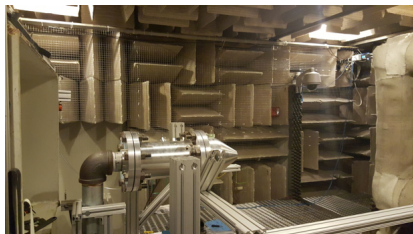
Figure 14: University of Florida Unsteady Fluid Dynamics Group Anechoic Chamber with installed nozzle for studying jet turbulence and acoustics.
