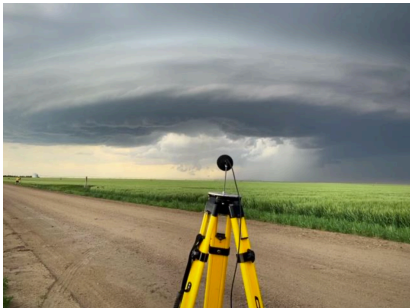
Figure 16: Infrasound microphone setup at tornado formation location on June 8th at c. 7:30 CDT.
