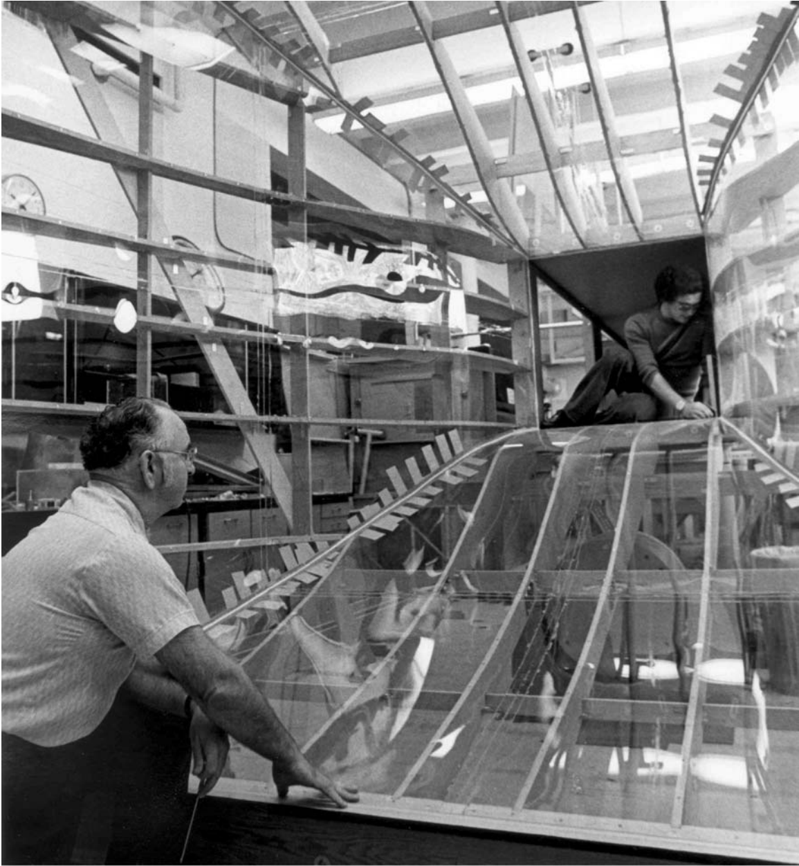
Figure 7. Bernie Leadon and student constructing a wind tunnel for studying wind loads on buildings.
